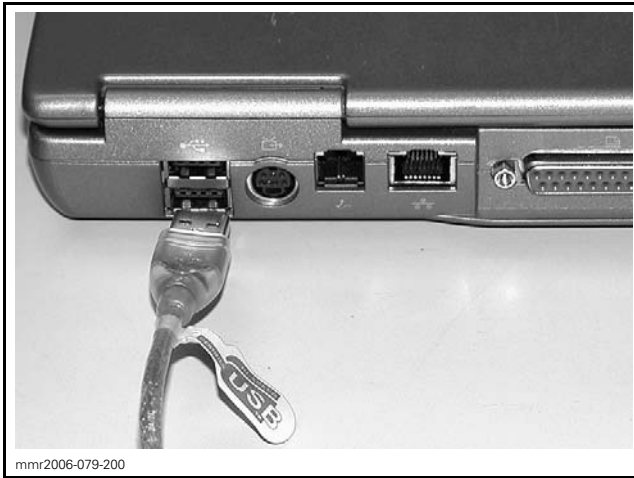
MPI-2 INTERFACE CARD CONNECTED TO USB PORT
